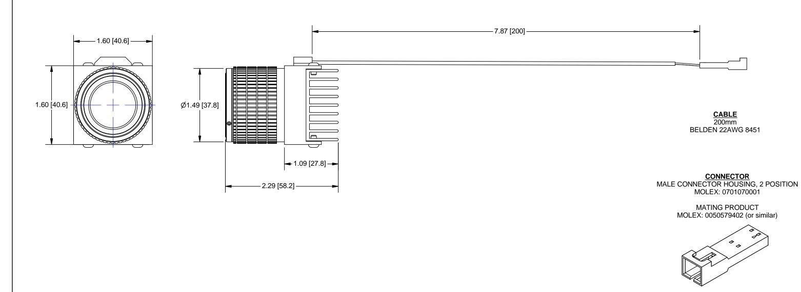
Pin 1- Anode Pin 2- Cathode
