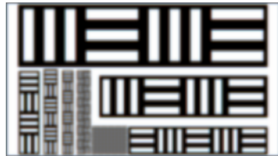
Resolv4K Zoom @ 4.5X High Mag 8.9MP Sensor – 0.76µm / pixel 3.56mm FOV – 5.20mm² Area (3.25X more)
